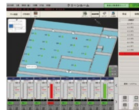
COD-203 Fixed-point monitoring based on installation drawings
