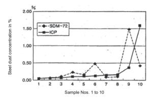
Figure A6. Concentration Comparison between SDM-72 and ICP
