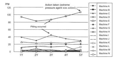
Figure A3. 5-year Steel Dust Concentration Trend in Lubricant Oil from Large-sized Speed Reducers
