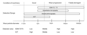
Figure A4. Iron Particle Diameter/Detection Range Comparison
